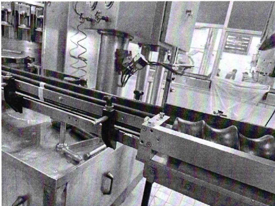
Image 3 Barcode reader (Cognex DataMan 290) mounted at the filler/capper outfeed for product/SKU detection
