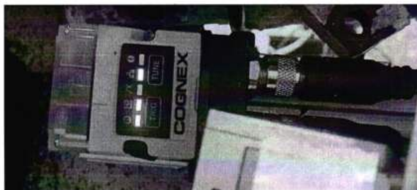
Image 1 — The Vendor's Cognex DataMan fixed-mount barcode scanner installed at the scanning point
