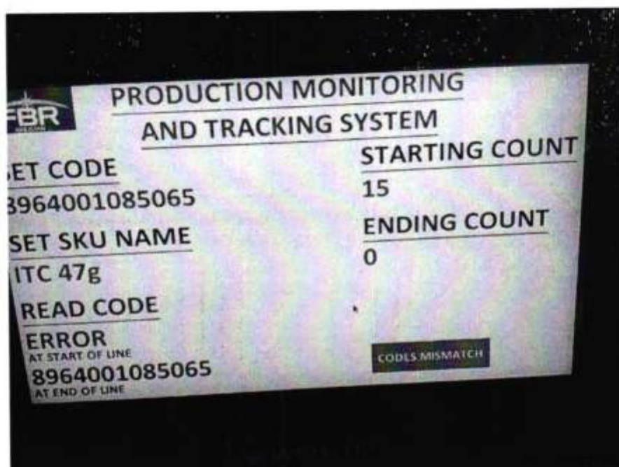
Image 6 — On-site display after Test 2 — pack count of 15 and 'Codes Mismatch' alert on cross-validation between start-of-line and end-of-line reads
