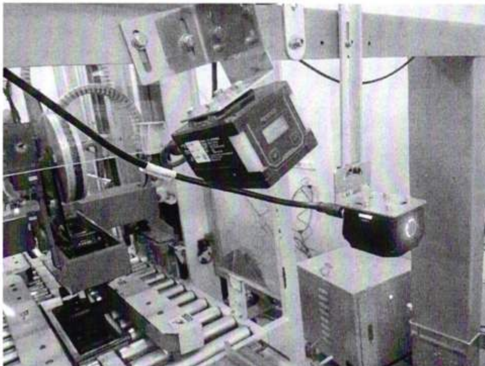
Image 2 — Inspection camera and fixed-mount code reader mounted on the gantry for stamp and carton-code reading
