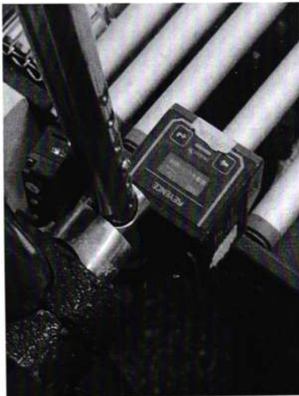
Image 1 — The Vendor's Keyence barcode reader and photoelectric counting sensor installed over the tea packing line conveyor
